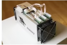
Application Specific Integrated Circuit (ASICs) 2013 – 2018 4 – 16 TH/S
